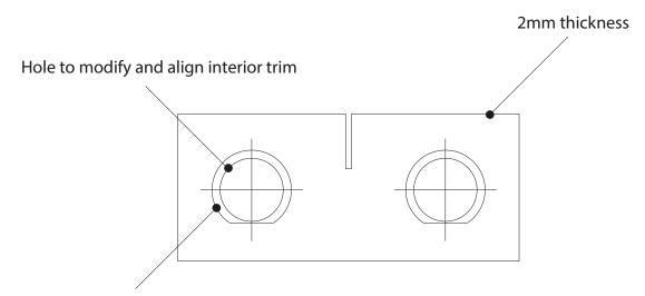
Hole to mount switch on backing plate
